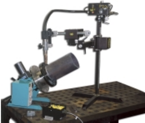
Application of FTS-1025 Automatic Height Control with Linear Weaver shown above.
